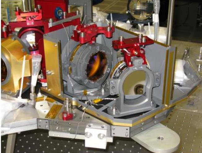
Figure 3: The NIRCcam flight unit in integration
