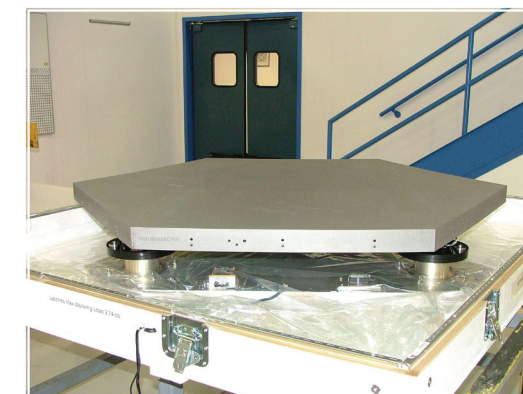
The uncoated front side of one of Webb's mirror segments. (AXSYS Technologies)
