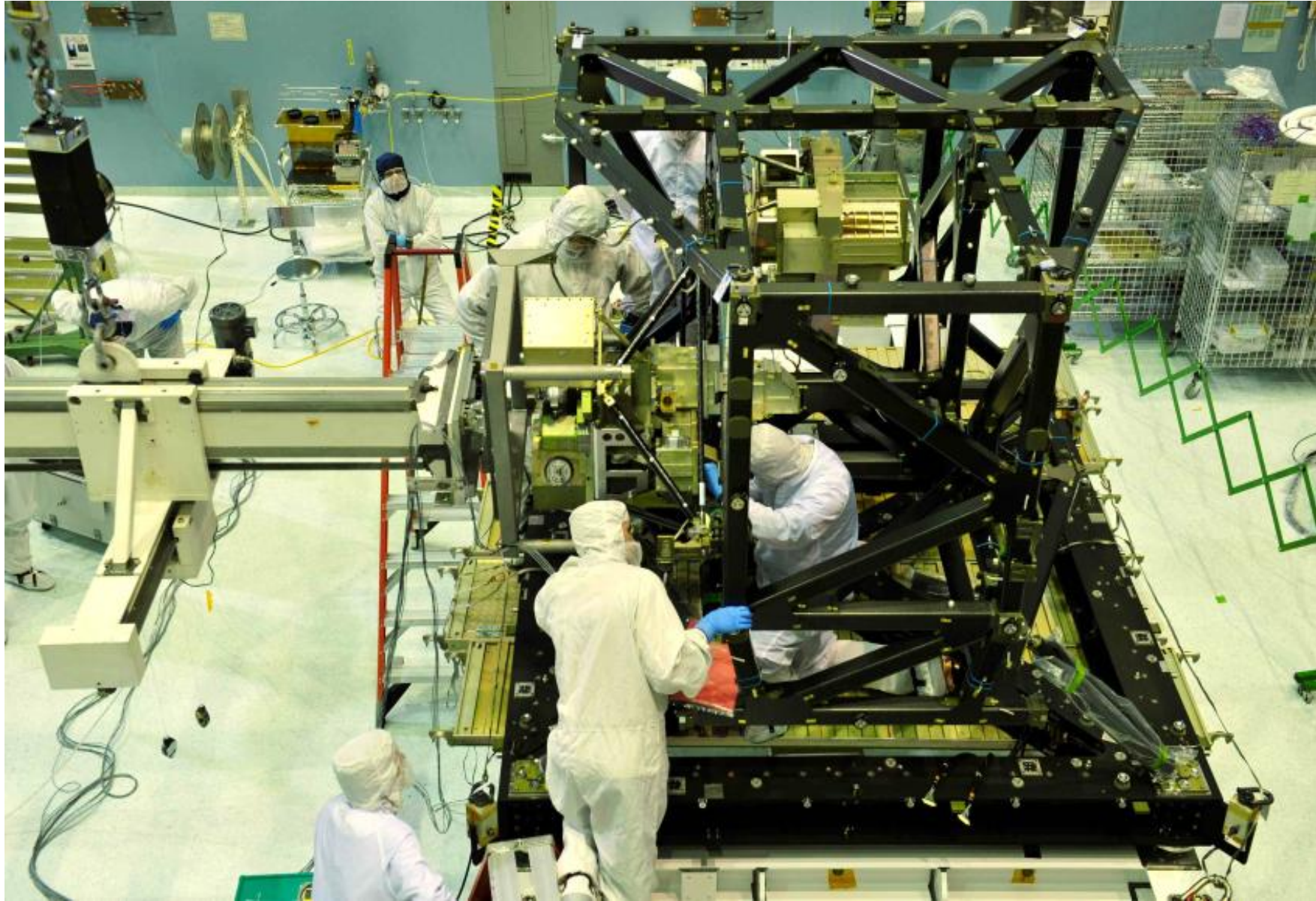
Test installation of MIRI Structural Thermal Model
