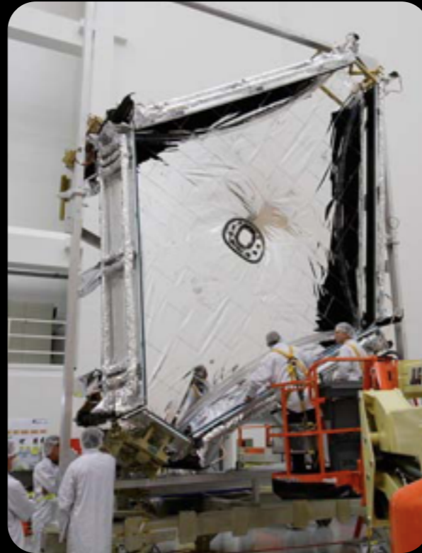
1/3rd scale thermal test
